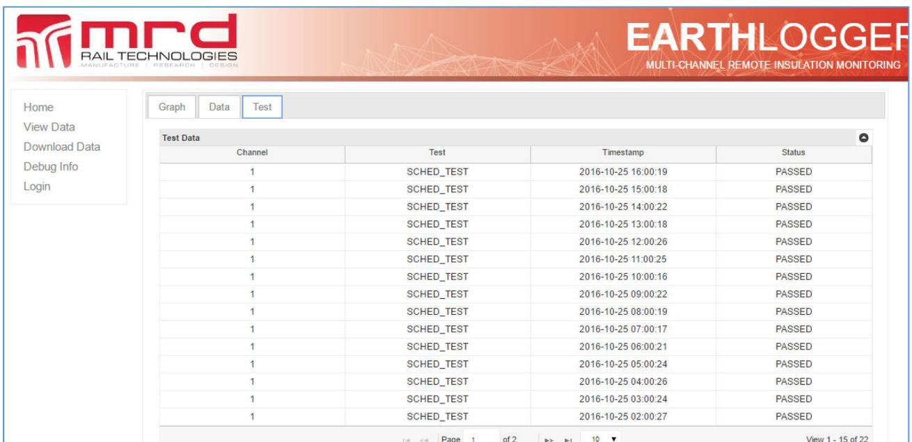
The screenshot shows the EarthLogger interface with the 'Test' tab selected. The 'Test Data' table is displayed with the following columns: Channel, Test, Timestamp, and Status. The table contains 16 rows of data. Below the table, there are navigation controls for 'Page 1 of 2' and a dropdown menu set to '10'. An 'export log data' button is located at the bottom left of the table area.
